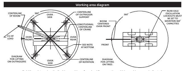
Bold lines determine the limiting position of any load for operation within working areas indicated.
