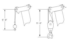
Dimensions are for largest Grove furnished hook block and headache ball, with anti-two block activated.
